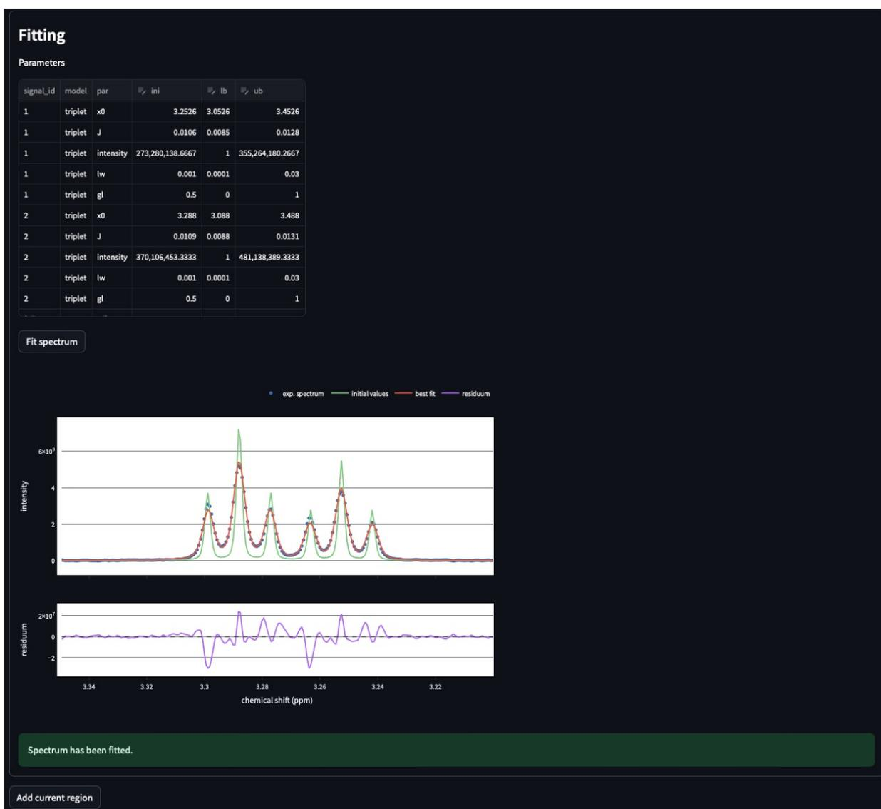
The fitted reference spectrum will be automatically displayed on the resulting graph. This plots will show [i] the experimental data as dots [ii] the best fit as red a curve and [iii] the initial values used in the minimization in green. This is supplemented with the residuum plot below.
